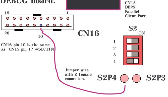
Turn ON S2 pin 4 to ground CN 16 pin 10 & CN15 pin 17 The software will then select to reprogram the serial EEPROM.. You supply the default IP address you want to use and the last two digits of the MAC Address ( between 0x50 - 0xFF)
